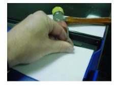
6. Place the hasp assemblies over the mounting holes. Obtain the four ¼-20x1 ¾ (long) Carriage Bolts and insert into the upper hasp assembly and mounting holes on the cabinet. Obtain the four 1/4 –20x1/2 (short) Carriage Bolts and insert into the lower hasp and mounting holes on the door. Remove all tools and hardware from top of Vender. Clean any debris and drill shavings from top of Vender. Carefully dismount ladder.
